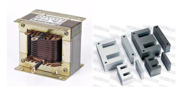
(1) Hot Rolled Silicon Steel Sheet for Electrical components (GB5212-85) Hot Rolled Silicon Steel Sheet for Electricity production is made of soft magnetic ferrosilicon alloy with low carbon loss, and hot rolled into a sheet with a thickness of less than 1mm. Hot rolled silicon steel sheet can be divided into low silicon (Si ≤ 2.8%) and high silicon (Si ≤ 4.8%).
