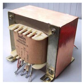
As we know, the actual transformer is always working in AC state, the power loss is not only from the coil resistance, but also generated in the core under the magnetisation of alternating current. Usually the power loss in the iron core is called "iron loss", iron loss caused by two reasons, one is "hysteresis loss", one is "eddy current loss".
