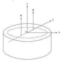
When the transformer is operating, there is an alternating current in the coil, which produces a magnetic field that is of course alternating. This varying magnetic field produces an inductive current in the iron
